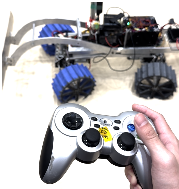
Figure 1: F710 joystick teleoperating our rover
