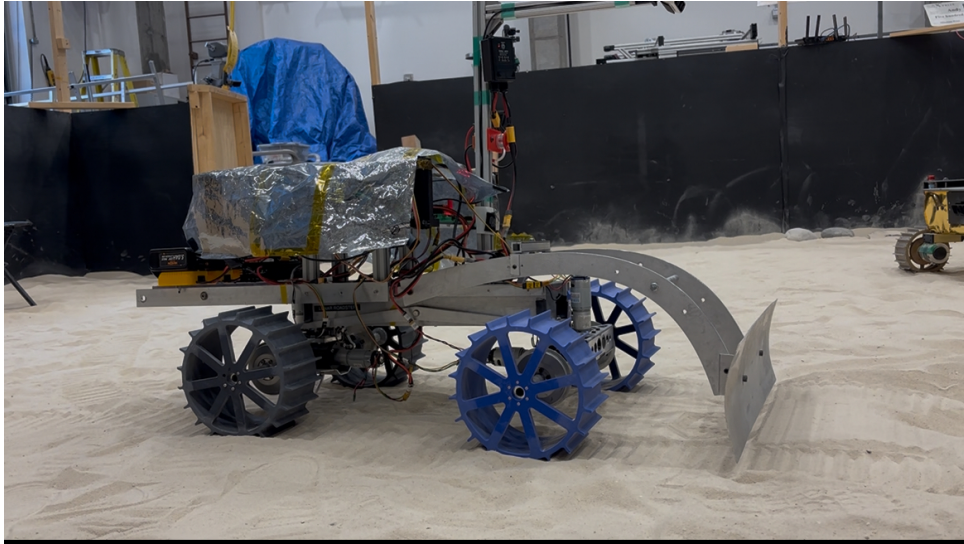
Figure 2: 4 printed wheels mounted on the rover
