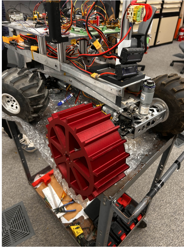
Figure 3: 3D printed wheel mounted on the ROADSTER
