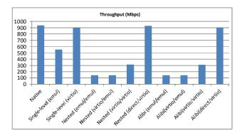
**Figure 6.** Performance of netperf in combinations of I/O virtualization methods between  $L_0/L_1$  and  $L_1/L_2$ . emul, virtio and direct refer to device emulation, para-virtualization and direct device assignment, respectively.
