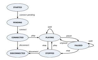
Figure 3: State machine for a connection process
