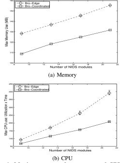
Figure 6: Maximum per-node memory and CPU usage across the network as number of NIDS modules grows. The total traffic volume is 100,000 sessions.
