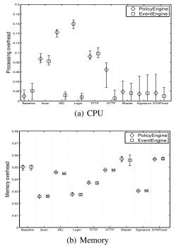
Figure 5: CPU and memory overhead for different modules with the coordination-enabled Bro prototype.
