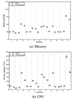
Figure 8: Memory and CPU load on each network node for 100,000 sessions and 21 NIDS modules.
