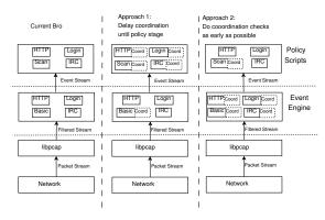
Figure 4: Implementing the coordination functionality in Bro. The "coord" boxes indicate where we add in coordination checks. For some modules (e.g., Scan), the checks have to be in the policy engine.
