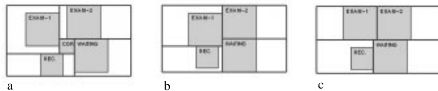
FIGURE 6. Removing the corridor in (a) with option ‘vertical’ (b) or ‘horizontal’ (c)
