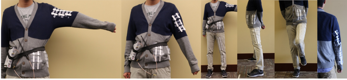
Fig. 8. RF-Wear prototype on body. We implement RF-Wear on OmniID IQ 150 tags attached to clothing and an Impinj Speedway RFID reader connected to a single-antenna. The tags are attached to fabrics of different material (a sweater is shown here) and on different body parts (around the knee, elbow, shoulder) the angles of these joints are tracked.
