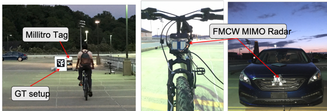
Figure 15: Millimetro was tested in 3 mobile environments: walking, biking and driving.
