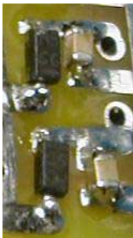
Figure 4-1: Power Supply Rectifier Implementation
