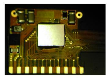
Figure 4. Retinal implant circuit board. The controller IC, as well as power supply and signal conditioning components, are inserted into the curved hermetic titanium case.
