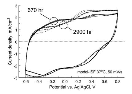
Figure 6. Cyclic voltammograms of eight SIROF electrodes after 670 hr (solid) and 2900 hr (dashed) of pulsing at 200  $\mu$ C/cm<sup>2</sup>.
