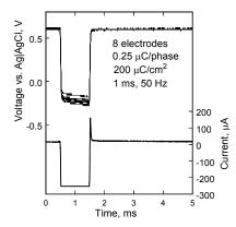
Figure 5. Voltage transients of eight SIROF electrodes on a polyimide array. The electrodes have been pulsed for 2900 hr at 200  $\mu$ C/cm<sup>2</sup>. A representative current waveform is also shown.
