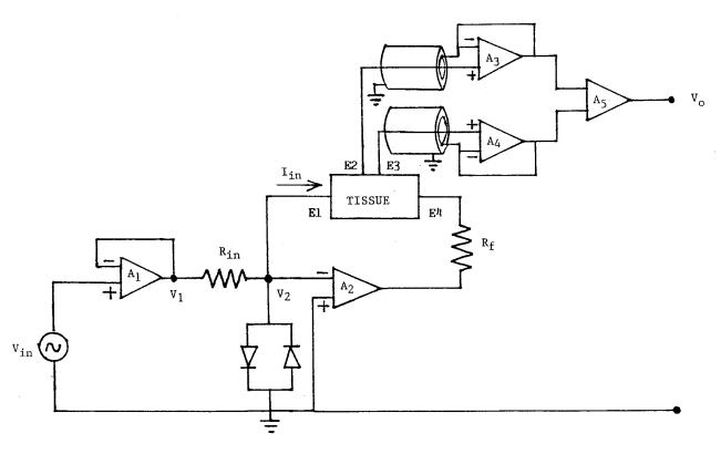
Fig. 2. The circuit for delivering current and measuring voltage across the conductivity cell. Constant current  $I_{\rm in}$  is generated in the lower portion of the circuit and fed across outer electrodes E1 and E4 of the four electrode array. Inner electrodes E2 and E3 are used to measure the resulting voltage difference across the sample.
