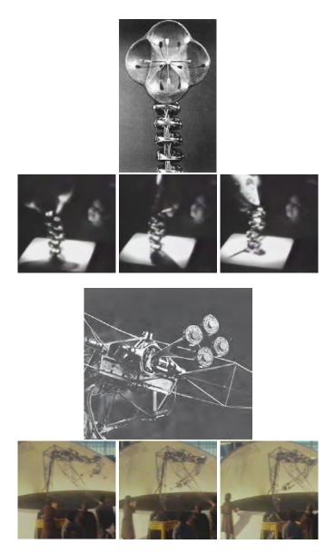
Ihnatowicz's S.A.M. – Sound Activated Mobile (top) and Senster (bottom) are one of the first robots to be designed as unique mechanical creatures.
