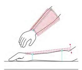
Image segmentation and touch detection are generated from the anatomy of the forearm. The medial axes of the arm create the 3D plane for segmentation. An offset from the 3D plane defines the 3D touch region of the forearm.
