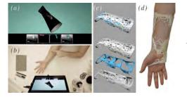
An arm brace designed using the generative manipulation mode. (a) skin input updates a touch heatmap of the user's forearm; (b) a design is generated using virtual agents; (c) resulting geometry is processed for fabrication; (d) the resulting physical artifact on the user.
