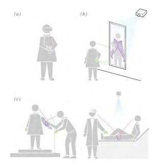
The point-of-view of the user or users determine the physical configuration of a skin-centric design tool: (a) firstperson systems have a direct line of sight to the user's canvas area, (b) second-person systems have partially occluded canvas areas, and (c) third-person systems enable multiple users to participate in design.
