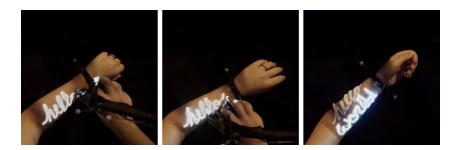
FIGURE 9 The user holds down the output button and extrudes over the rendered design.
