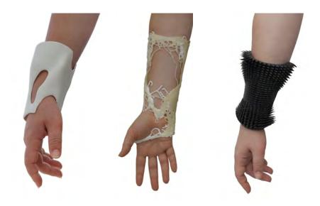
FIGURE 15 Artifacts developed with Tactum were verified by printing designs on FDM, SLS, and SLA 3D printers.
