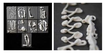
FIGURE 7 ExoSkin uses a water-based polymer clay as its printing medium.
