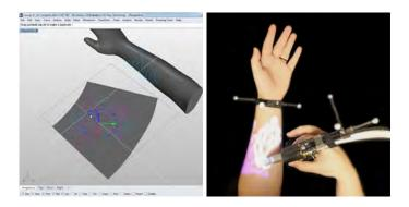
FIGURE 13 Designs in ExoSkin can be generated in commercial CAD software and then projected onto the body for fabrication.
