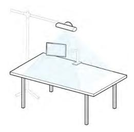
The initial workstation for Tactum was comprised of a Microsoft Kinect mounted above the work area to track user input, and Microsoft Surface tablet mounted within the work area to display visual output.
