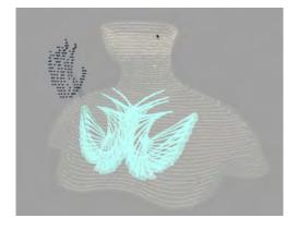
FIGURE 3 Reverb enables a designer to drape intelligent, fabrication-aware geometry around a 3D scan of their own body.
