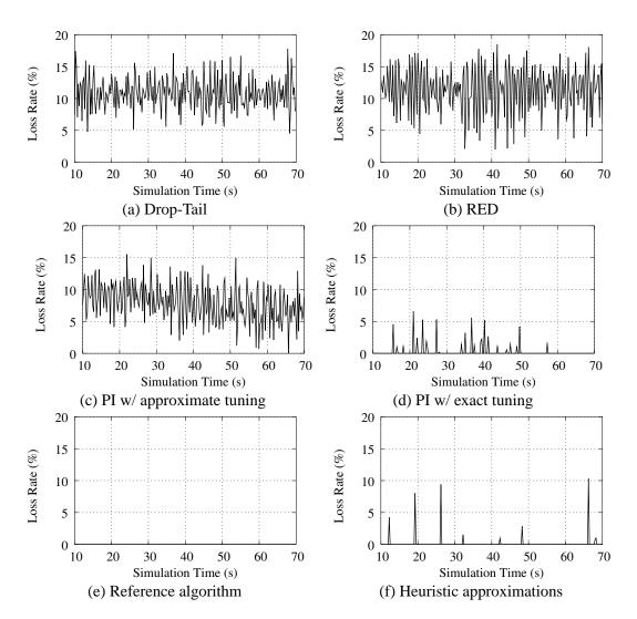
Figure 7.3: Loss rates. The figures compare the loss rates obtained with all six algorithms. Note that the reference algorithm does not discard any traffic.
