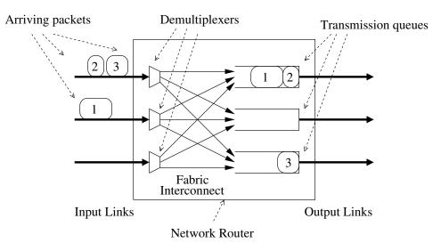
Figure 3.1: **Router architecture.** In this dissertation, we consider an output-queued router, where all queueing occurs at the output links, in the transmission queues. There is no contention at the input links or in the fabric interconnect. The figure shows a  $3 \times 3$  switch.
