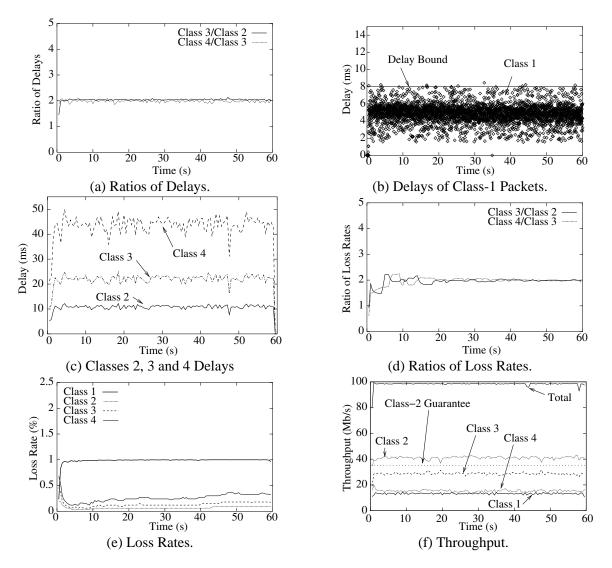
Figure 6.8: **Experiment 1: Router 2.** The graphs show the service obtained by each class at the output link of Router 2.
