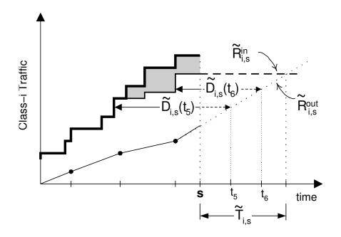
Figure 3.3: **Predicted input curve, predicted output curve, and predicted delays.** The prediction is performed at time *s* for the time interval  $[s, s + \tilde{T}_{i,s}]$ .
