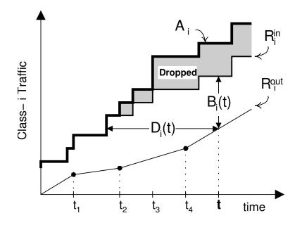
Figure 3.2: **Delay and backlog.**  $A_i$  is the arrival curve,  $R_i^{in}$  is the input curve and  $R_i^{out}$  is the output curve.
