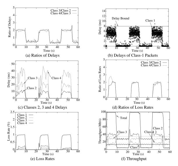
Figure 6.11: **Experiment 2: Router 2.** The graphs show the service obtained by each class at the output link of Router 2.
