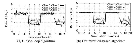
Figure 5.4: **Experiment 1: Delay differentiation.** The graphs show the proportional delay differentiation obtained by each class at the simulated 1 Gbps bottleneck link. (b) is a duplicate of Figure 4.4(a).
