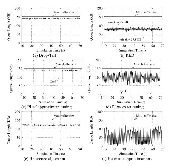
Figure 7.5: **Queue lengths.** The figures compare the queue lengths at the router for all six algorithms.
