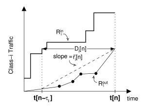
Figure 5.2: **Definition of the average rate**,  $\overline{r_i}$ . This figure shows the relationship between  $D_i[n]$ ,  $\tau_i$  and  $\overline{r_i}[n]$ .
