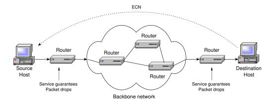
Figure 1.2: **Illustration of the deployment of the proposed service in a network.** Routers are in charge of transmitting and dropping packets according to the available resources and the QoS desired. Routers set the regulation signals (ECN), which are used by the end-hosts to regulate their traffic.
