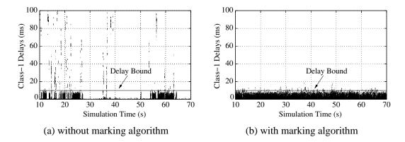
Figure 7.6: **Class-1 packet delays.** Note that the violations are much smaller in magnitude with the marking algorithm.
