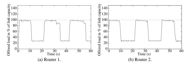
Figure 6.9: Experiment 2: Offered load. The graphs show the offered load at Routers 1 and 2.
