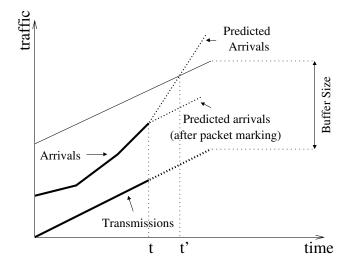
Figure 7.1: **Overview of the marking algorithm.** At time t of a packet arrival, the router predicts future arrivals, by inferring how the TCP source will send traffic. When an impending buffer overflow is predicted, at time t' here, a packet is marked to reduce future arrivals.
