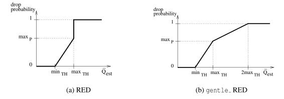
Figure 2.1: **Drop probability in RED.** The probability of dropping a packet is a function of an estimate on the average queue size in RED and gentle\_RED.
