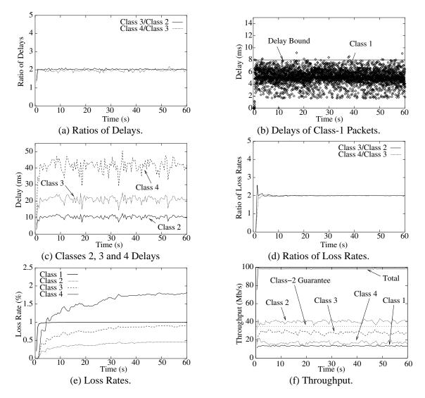
Figure 6.7: **Experiment 1: Router 1.** The graphs show the service obtained by each class at the output link of Router 1.
