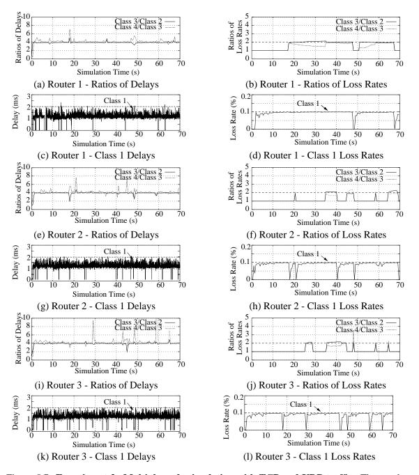
Figure 5.7: **Experiment 2: Multiple node simulation with TCP and UDP traffic.** The graphs show the delays and loss rates encountered at each router by Class 1 traffic, and the ratios of delays and the ratios of loss rates for Classes 2, 3 and 4 at each router. The absolute constraints and the target ratios are indicated by straight dashed lines.
