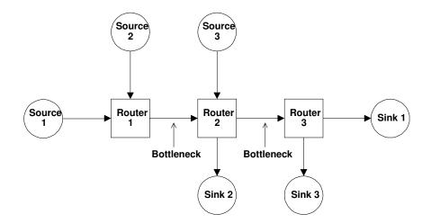
Figure 6.5: **Experiments 1 and 2: Network topology.** All links have a capacity of 100 Mbps. We measure the service provided by Router 1 and 2 at the indicated bottleneck links.
