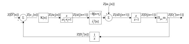
Figure 5.3: **The class-***i* **delay feedback loop.** This model uses *z*-transforms of the relationships derived in Section 5.2.2.
