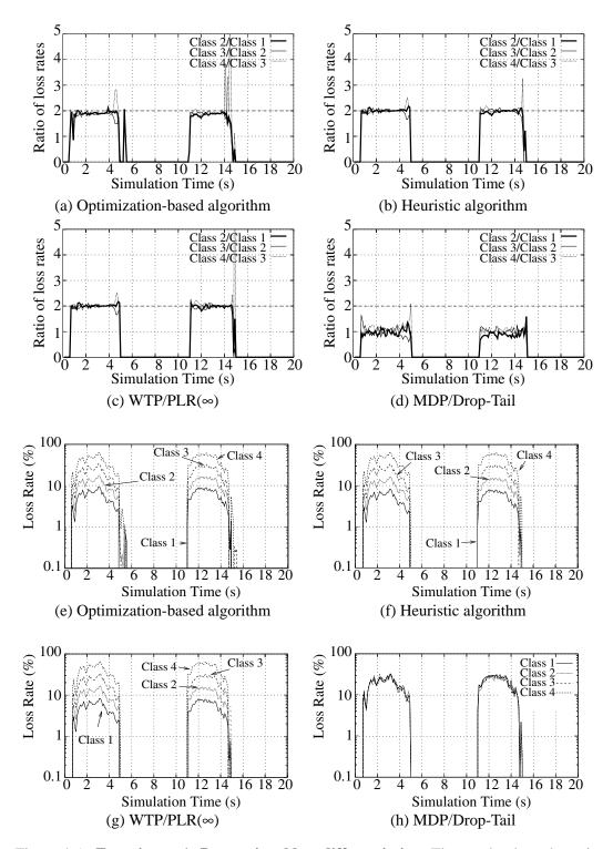
Figure 4.5: Experiment 1: Proportional loss differentiation. The graphs show the ratios of loss rates for successive classes (a)-(d) and the loss rates (e)-(h). The target value for the ratios, indicated by a dashed line, is k' = 2.
