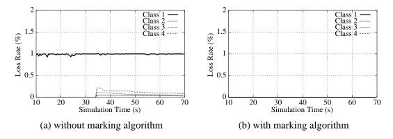
Figure 7.7: Loss rates. The marking algorithm prevents any traffic from being dropped.
