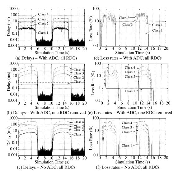
Figure 4.6: **Experiment 2: Delay and loss differentiation.** The graphs show the delays of all packets in (a)-(c) and the loss rates of all classes in (d)-(f). All results are for the heuristic algorithm.
