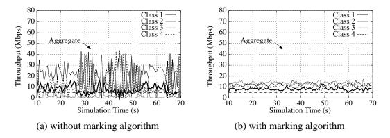
Figure 7.8: **Per-class throughputs.** Without the marking algorithm, we observe oscillations and sporadic violations of the Class-1 throughput guarantee. The marking algorithm stabilizes these oscillations and ensures the throughput guarantees are respected.
