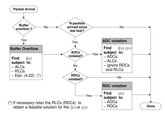
Figure 4.2: **Outline of the heuristic algorithm.** The heuristic algorithm decomposes the optimization problem into several smaller, computationally less intensive, problems.
