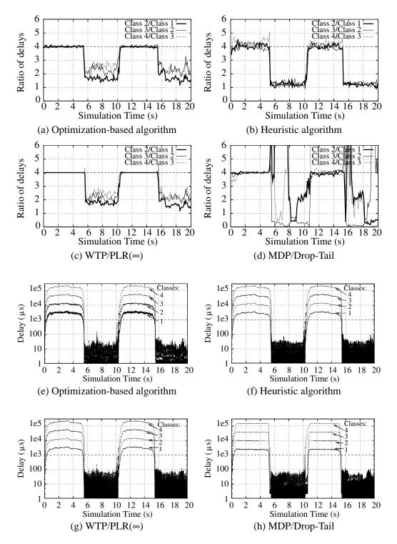
Figure 4.4: **Experiment 1: Proportional delay differentiation.** The graphs show the ratios of the delays for successive classes (a)-(d) and the absolute delay values (e)-(h). The target value for the ratios, indicated by a dashed line, is k = 4.
