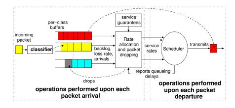
Figure 6.2: Architecture of an output queue in the QoSbox. The three main components are the packet classifier, in charge of storing incoming packets in the proper FIFO per-class buffer, the rate allocation and dropping algorithm, and the scheduler, which forwards packets according to the service rates allocated.
