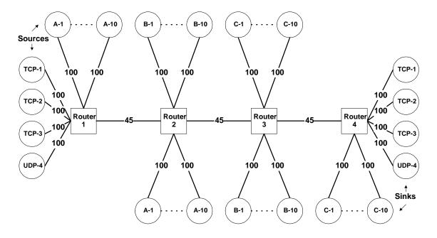
Figure 5.6: **Experiment 2: Network topology.** The labels of the links denote the links capacities in Mbps.
