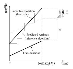
Figure 7.2: Linear interpolation. In the heuristic, only the value  $\widetilde{R}_{t}^{in}(t + \max_{i} \{\tau_{i}\})$  is computed, and is used to determine the excess traffic that will arrive at the router.
