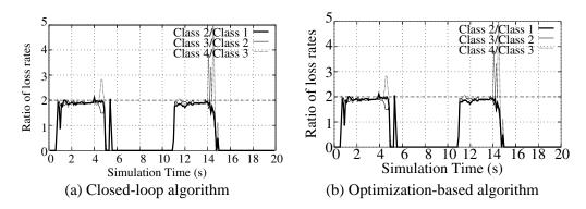
Figure 5.5: **Experiment 1: Loss differentiation.** The graphs show the proportional loss differentiation obtained by each class at the simulated 1 Gbps bottleneck link. (b) is a duplicate of Figure 4.5(a).
