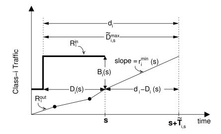
Figure 4.1: **Determining service rates required to meet delay bounds.** The figure indicates the service rate  $r_i^{\min}(s)$  required so that the maximum predicted delay satisfies  $\widetilde{D}_{i,s}^{max} = d_i$ . Allocating at least  $r_i^{\min}(s)$  ensures that the delay bound  $d_i$  is met for class *i*.
