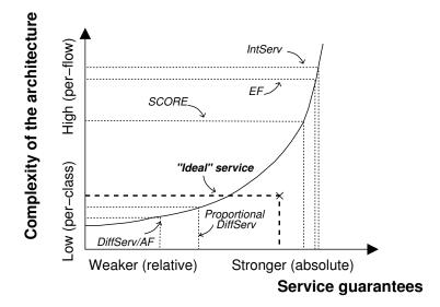
Figure 1.1: The trade-off between strength of service guarantees and complexity of the implementation. IntServ and Expedited Forwarding provide very strong service guarantees at the cost of per-flow complexity, while Assured Forwarding only provides limited service assurance, but has low complexity. Ideally, a service should be able to provide strong service differentiation with low complexity. Note that the picture is qualitative.
