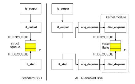
Figure 6.3: Functions and structures associated with the output queue in BSD and ALTQenabled BSD. Each queueing discipline implemented in ALTQ consists of a kernel module, represented by the dotted box.
