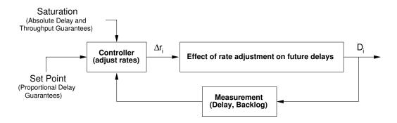
Figure 5.1: **Overview of the closed-loop algorithm.** The figure is an overview of the feedback loop for delay differentiation. A similar mechanism is used for loss differentiation.
