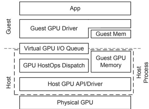
Figure 3: GPU Paravirtualization Architecture.
