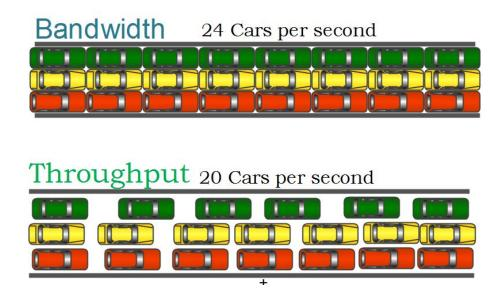
Fig1. Difference between throughput and bandwidth
