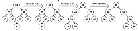
Finish the code below for splay tree insertion, using the rotation functions discussed in class:
