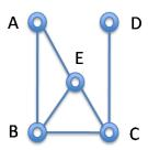
and the goal to find a path from E to B. Let's say we start E-C and then C-D. At this point, all the vertices we could go to (which is only C) have already been marked! So we have to *backtrack* to the most recent choice point and pursue alternatives. In this case, this could be C, where the only remaining alternative would be B, completing the path E-C-B. Notice that when backtracking we have to go back to C even though it is already marked.
