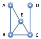
We can go  $A - B - E - A - B - E - \cdots$  without ever reaching D (or we can go just  $A - B - A - B - \cdots$ ), even though there exists a path.
