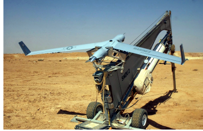
(a) ScanEagle 3m wingspan 13kg empty
