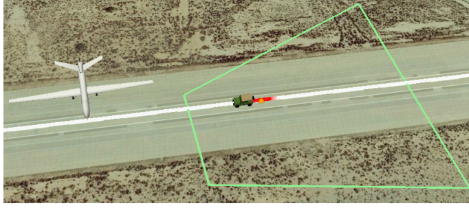
Figure 4.20: Visualization example from simulation showing a UAV pursuing a Jeep. The green trapezoid is the ground region visible to the camera. The orange dot indicates the geolocation filter's best estimate of the target's position at the center of the red smear denoting the surrounding uncertainty distribution.
