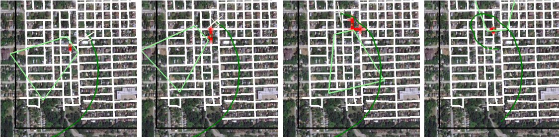
Figure 4.22: An example of pursuit in a road network using cellular decomposition. The UAV anticipates loss of view (area within the green trapezoid) and begins to turn sharply. While out of view, it predicts diffusion in possible target location (red probability mass) and greedily steers to maximize the probability of re-detection.
