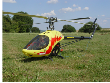
(b) Joker 2 1.8m rotor diam. 8kg loaded
