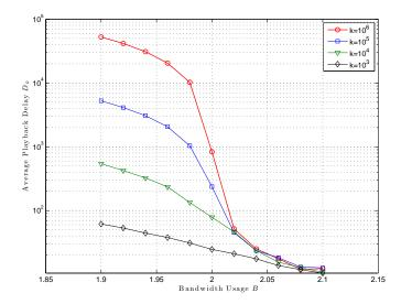
Fig. 2. The bandwidth-delay trade-off for different values of stream length k, and  $\epsilon=0.5$ . This figure shows the transition in the behaviour of playback delay at  $B=\frac{1}{(1-\epsilon)}=2$ .
