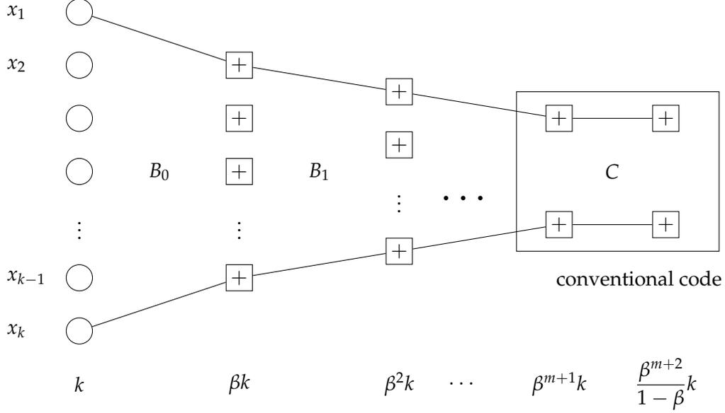
Figure 1: A visualization of a Tornado code. The  $k$  information symbols are inputted into a cascade of  $k$  sparse bipartite graphs and a conventional code. The output of the Tornado code is the  $k$  information symbols and the  $n - k$  parity check symbols.
