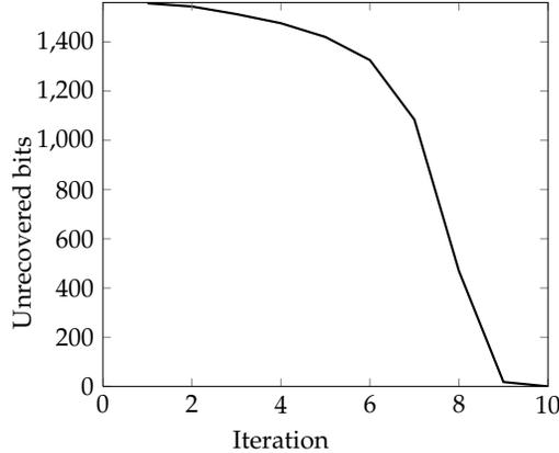
Figure 13: Number of bits still erased versus decoder iteration number for  $k = 16,000$ ,  $n = 32,000$  and  $p = 0.1$ . We observe the Tornado effect in that the algorithm struggles for most of the run and quickly converges to the solution in a very short number of runs.
