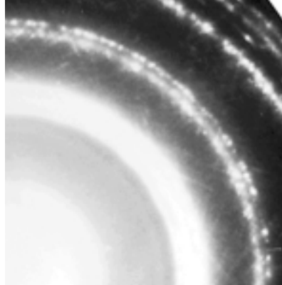
Fig. 2.19 Electron diffraction pattern of a CoCrPtTa film in (11.0) texture. The streaks are due to the SFs [169] (© 2000 IEEE).
