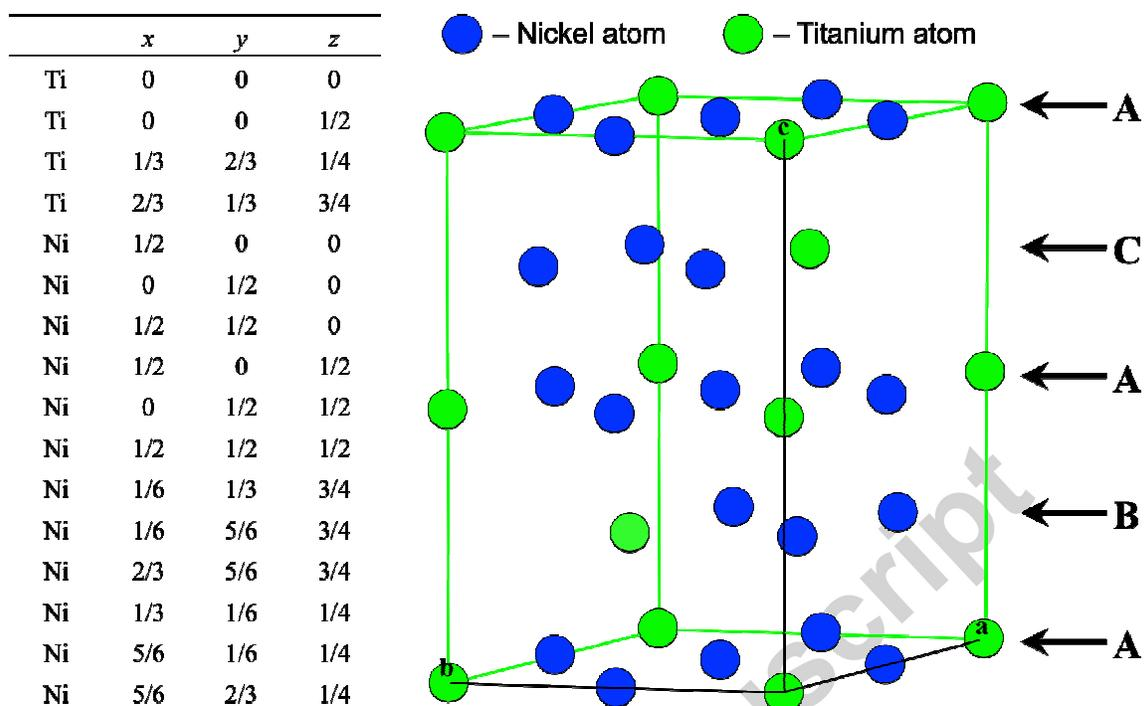
Fig. 7 The unit cell of the  $\eta$ -Ni<sub>3</sub>Ti phase and a complete list of the 16 sites of the unit cell.
