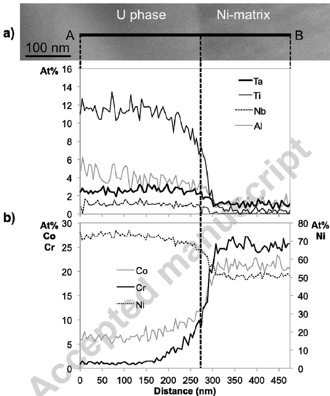
Fig. 6 a) The high-angle-annular-dark-field STEM micrograph of the U phase/Ni-matrix phase boundary. An elemental line profile was acquired along line AB using EDS with a step size of 5 nm. b) The corresponding quantified elemental line profile. The elements that were included in the quantification were: Ni, Ti, Ta, Co, Cr, Nb and Al.
