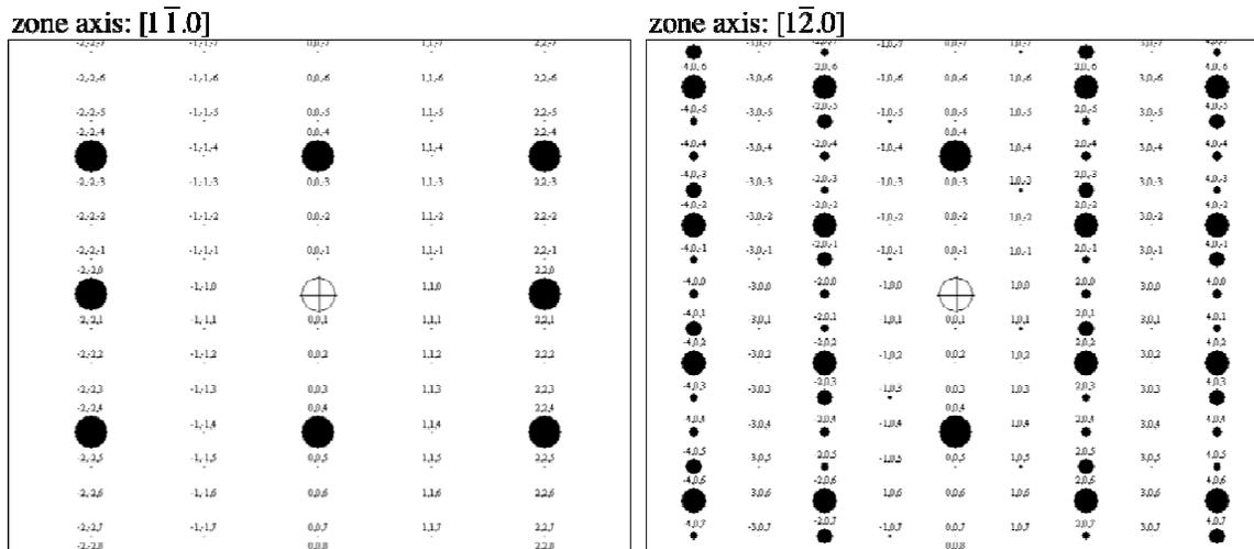
Fig. 9 Simulated  $[1\bar{1}0]$  and  $[1\bar{2}0]$  zone axis diffraction pattern for substitution of any one of the 16 sites in the unit cell of  $\eta$  phase by a Ta atom. (The spots that are labeled by plane indices are the ones allowed for the structure)
