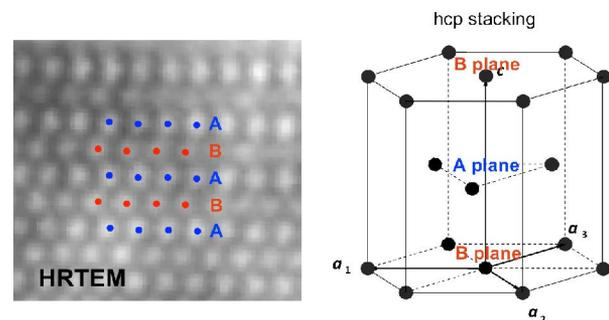
Fig. 1. High-resolution TEM and schematic illustration of the hcp structure.
