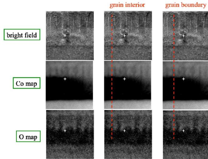
Fig. 2. EFTEM BF image of Co-alloy + oxide media and EELS elemental maps of Co and O elements (the same area).
