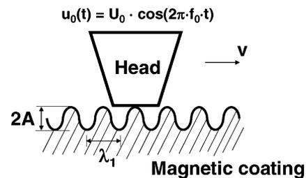
Fig. 1. Schematic of a head–medium interface. A magnetic head is in contact with a coating surface of which the contour varies sinusoidally.
