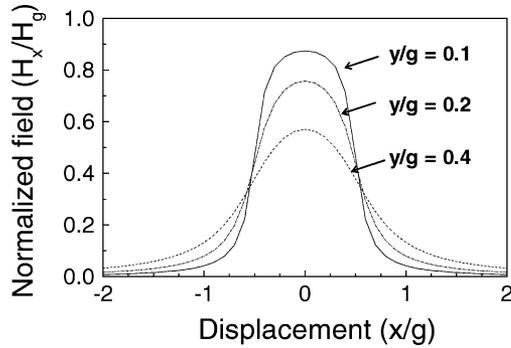
Fig. 6. Normalized Karlqvist head field  $H_x$  for different head-to-tape spacing. With a smaller spacing, a sharper write field gradient can be seen by the recording medium.
