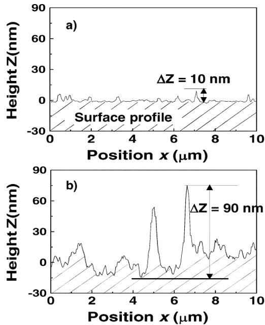
Fig. 10. Typical surface profiles for media A and B measured by AFM. The maximum vertical distance  $\Delta z$  for medium A is 10 nm while  $\Delta z$  of 90 nm is observed for medium B. (a) Medium A. (b) Medium B.
