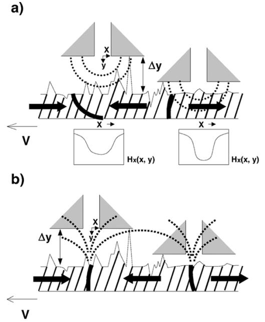
Fig. 3. Illustration of (a) transition broadening and (b) output loss, resulting from surface roughness. Peak asperity lifts the head away from the tape, resulting in spacing fluctuation  $\Delta y$ .  $H_x(x, y)$  represents the  $x$  component of the head field produced by a write head.
