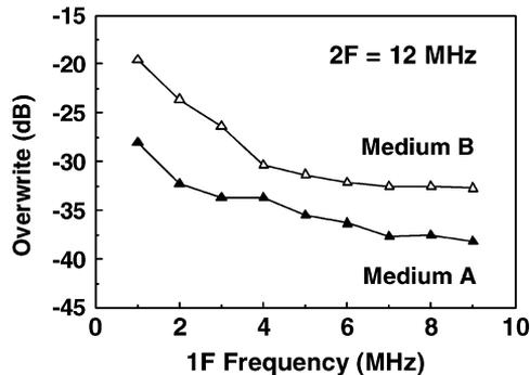
Fig. 11. Overwrite performance for media A and B as a function of the overwritten frequency (1F). The overwriting frequency (2F) is 12 MHz ( $\lambda = 0.56 \mu\text{m}$ ). For medium A, about 5 dB higher values over the whole frequency range were obtained.
