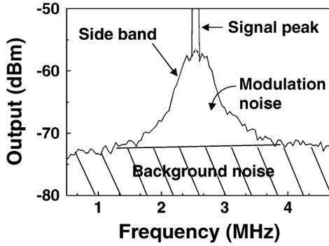
Fig. 2. Typical modulation noise spectrum from readback. Shaded area is the integrated background noise.
