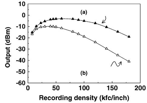
Fig. 8. Dependence of the reproduced output on the substrate roughness. The roughness ( $R_a$ ) of the sputtered media on (a) smooth PEN substrates is 1.3 nm while 6.1 nm on (b) conventional PEN substrates.
