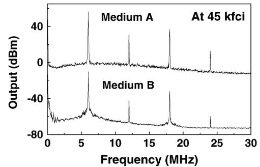
Fig. 4. Spectrum of 45 kfc/in density signal for media A and B. Use of smooth substrates significantly reduced modulation noise about the carrier frequency. Medium A is nearly free of modulation noise while for medium B, the sidebands of the fundamental component are clearly visible.
