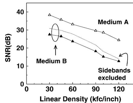
Fig. 5. SNR with increasing recording density for sputtered tape media A and B. The dotted line presents the change in SNR for sputtered tape medium B when the sidebands are excluded during SNR computation.
