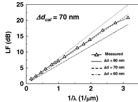
Fig. 9. Measured output difference, loss factor (LF) as a function of wavelength ( $\lambda$ ) for media A and B. The mean head-to-tape spacing difference  $\Delta d_{cal}$  for the two was obtained by a best fitting.
