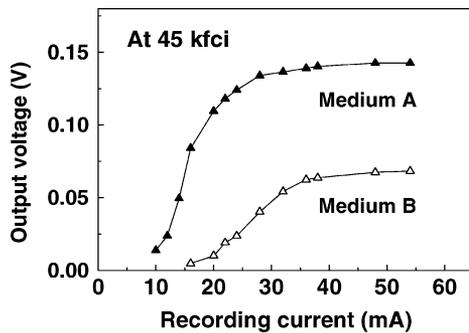
Fig. 7. Saturation curves for media A and B with respect to recording current at linear density of 45 kfc/i. The lower head-to-tape spacing for medium A led to a better saturation characteristic.
