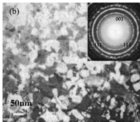
FIG. 1. (a) XRD patterns and (b) bright field image and SAD patterns for (a) FePdPt 20 nm/(on oxidized Si substrate) after RTA process for 30 min.
