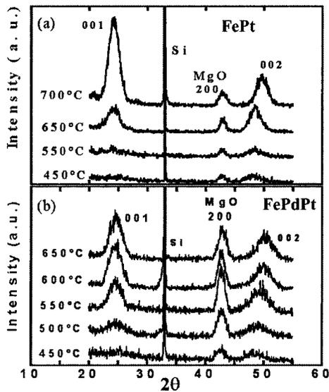
FIG. 2. XRD patterns after RTA process for 10 min at various temperatures (a) for FePt 5 nm films/MgO 10 nm and (b) for FePdPt 5 nm / MgO 10 nm films.
