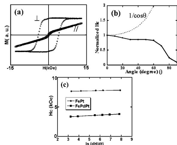
FIG. 4. (a) Hysteresis loops and (b) angular dependence of coercivity for FePdPt 5 nm/MgO 10 nm films after RTA at 650°C for 18 min. Angle is defined between the magnetic field and perpendicular direction to film plane (c) Coercivity vs field sweep rate for the fully ordered FePt 5 nm/MgO 10 nm and FePdPt 5 nm/MgO 10 nm films, annealed (RTA) at 700 and 650°C for 18 min, respectively.
