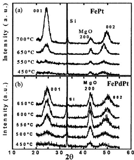
FIG. 2. XRD patterns after RTA process for 10 min at various temperatures (a) for FePt 5 nm films/MgO 10 nm and (b) for FePdPt 5 nm / MgO 10 nm films.
