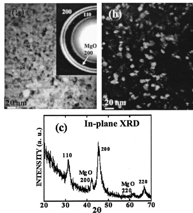
FIG. 3. (a) SAD patterns, bright field (BF), (b) dark field (DF) images and (c) in-plane XRD spectra ( $\theta/2\theta$  scan with grazing incidence beam of 2°) for FePdPt 5 nm/MgO 10 nm films after RTA at 650°C for 18 min.
