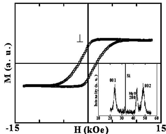
FIG. 5. Hysteresis loop (perpendicular to films) and XRD pattern (the inset figure) for *in situ* ordered  $5$  nm FePdPt films with an MgO underlayer ( $10$  nm) on Si substrate at  $530^\circ\text{C}$ .
