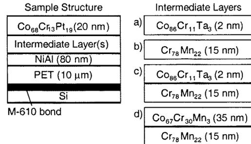
Fig. 1. Structure of the four complete stacks studied in this work. Each of the intermediate layers indicated (a)–(d) was inserted into the sample stack at the indicated location to form the four structures studied in this work. Partially complete versions of these samples were also examined.
