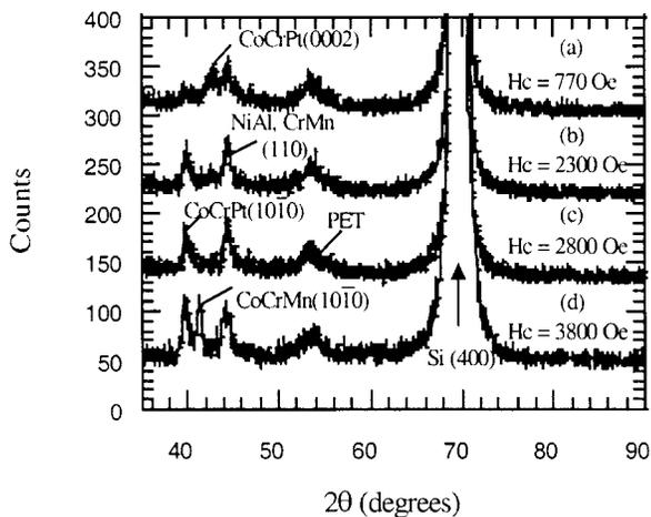
Fig. 2. XRD spectra of the four complete stacks. The textures and magnetic coercivities of these layers are strongly dependent on intermediate layers, as labeled in the figure. Refer to Fig. 1 for structure identities.
