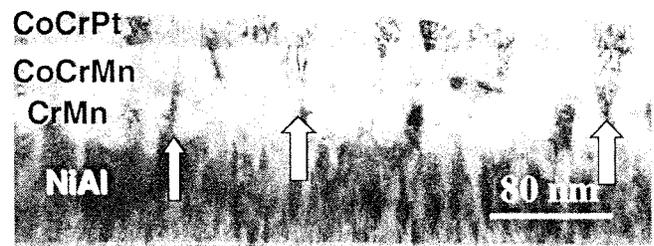
Fig. 4. Cross-sectional TEM image of NiAl/CrMn/CoCrMn/CoCrPt films (structure d). Although grain-to-grain growth penetrates all the layers (see arrows), the CoCrMn/CoCrPt interface shows better epitaxial growth.
