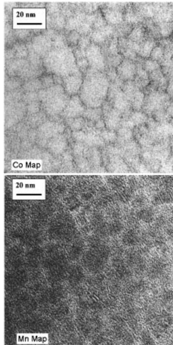
Fig. 5. The plane-view mapping image of Co and Mn concentration in the annealed CoPt film.
