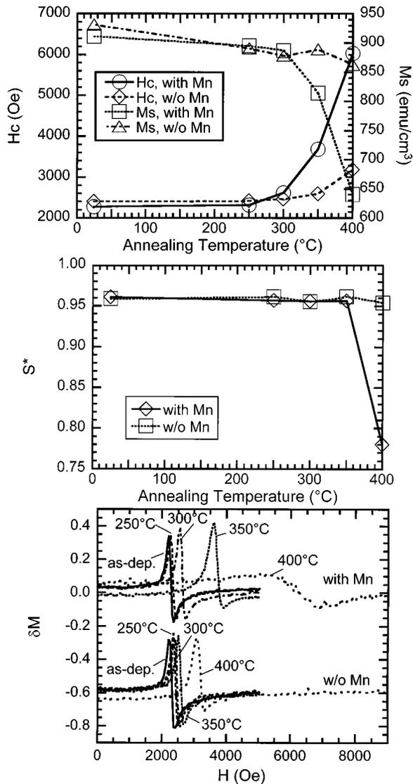
Fig. 1.  $H_c$ ,  $M_s$ ,  $S^*$ , and  $\delta M(H)$  curves as a function of the annealing temperature for the samples with and without the Mn layer.
