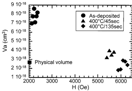
Fig. 3. Activation volume for as-deposited and annealed films.
