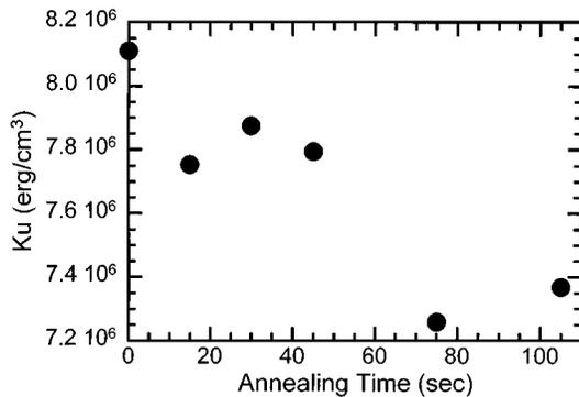
Fig. 4. Anisotropy constant versus annealing time at the temperature of 400°C.
