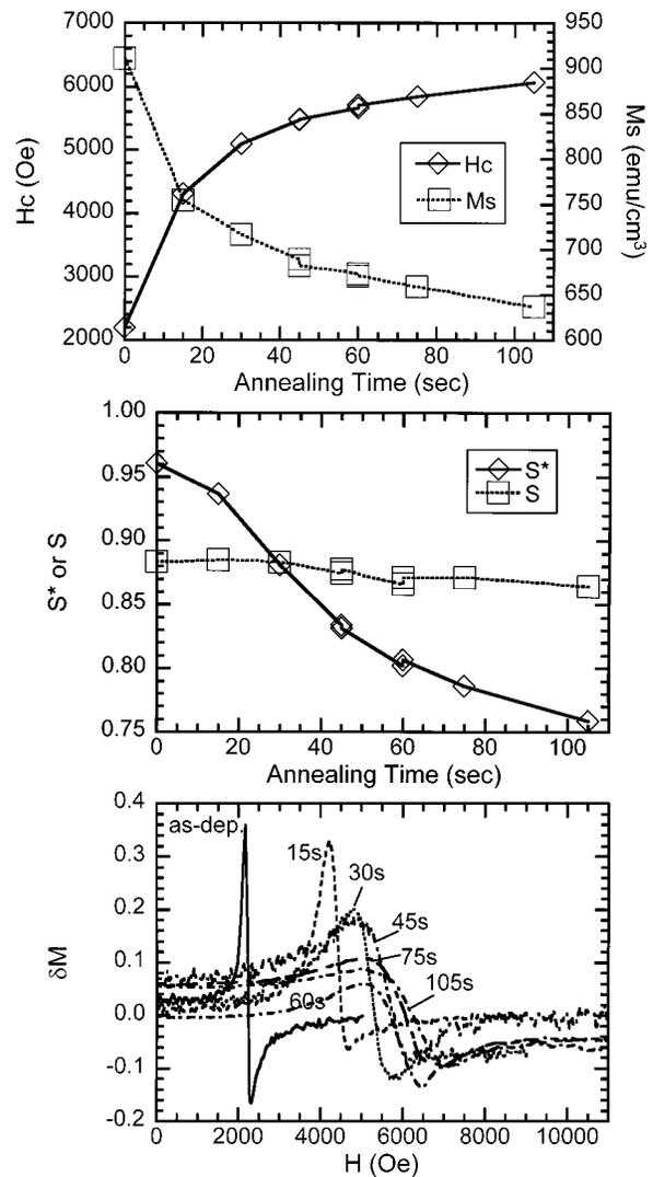
Fig. 2.  $H_c$ ,  $M_s$ ,  $S^*$ ,  $S$ , and  $\delta M(H)$  curves as a function of the annealing time at 400°C for the sample with the Mn layer.
