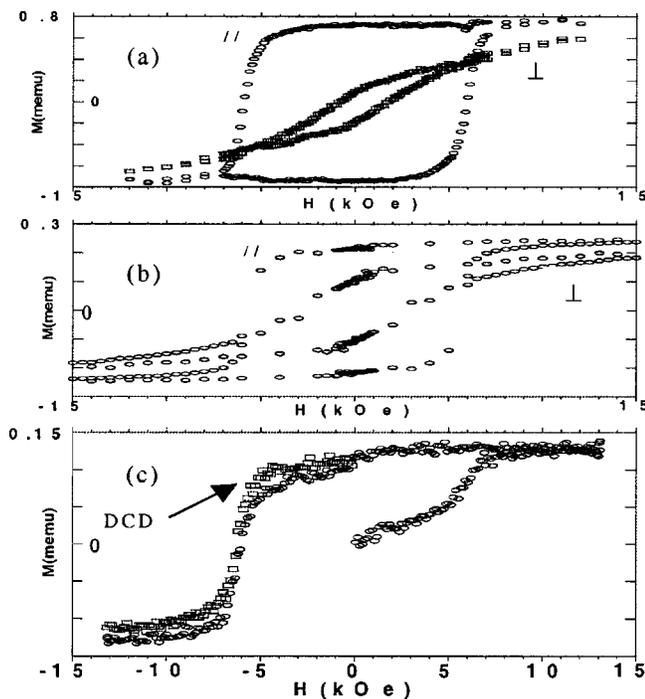
FIG. 4. Hysteresis loops for (a) 40 nm CoPt/10 nm MgO; (b) 40 nm CoPt/40 nm MgO after 8 min of RTA at 650 °C; (c) initial and demagnetization curve after ac demagnetization for 20 nm CoPt/40 nm MgO films, in-plane direction, 8 min of RTA at 650 °C.
