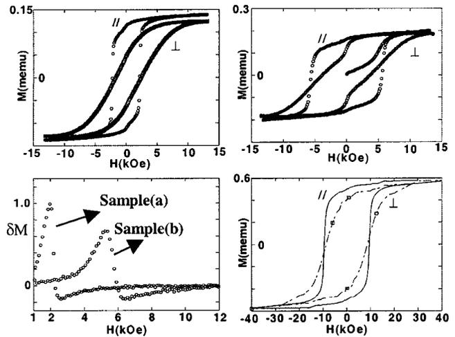
FIG. 3. Hysteresis loops for 40 nm CoPt/40 nm Ag/40 nm MgO films annealed at (a) 600 °C (8 min of RTA); (b) 650 °C (8 min of RTA), including initial magnetization after ac demagnetization in plane direction; (c)  $\Delta M$  of samples (a) and (b); (d) 700 °C, 8 min of RTA.
