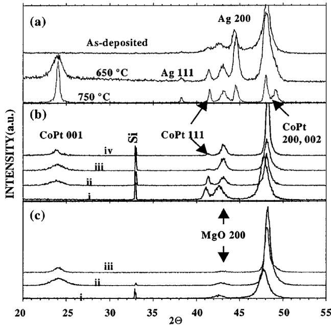
FIG. 1. XRD spectra for (a) CoPt 40 nm/Ag 40 nm/MgO 40 nm (8 min of RTA); (b) CoPt (20,40) nm/MgO 40 nm (8 min of RTA). From the bottom are (i) as-deposited 40 nm CoPt, (ii) annealed at 650 °C, (iii) 20 nm CoPt annealed at 650 °C, and (iv) 20 nm CoPt annealed at 750 °C; (c) CoPt 40 nm/MgO 10 nm (8 min of RTA), (i) as-deposited films, (ii) films annealed at 650 °C, and (iii) films annealed at 750 °C.
