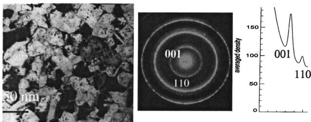
FIG. 2. Bright field image and SAD patterns of a 40 nm CoPt/10 nm MgO film after 8 min of RTA at 650 °C. Radial function of average peak intensity was mapped from SAD patterns by an IDL routine.
