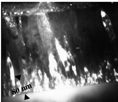
Figure 4 NiAl (110) Dark field image showing that most of the (110) oriented grains are near the film substrate interface.
