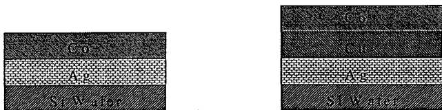
Fig. 1 Schematic drawing of the Co film structures epitaxially grown on Si wafers.
