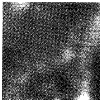
Figure 4. MFM 40\ \mu\text{m} \times 40\ \mu\text{m} images taken on \text{Fe}_{44}\text{Co}_{44}\text{Zr}_7\text{B}_4\text{Cu}_1 alloy ribbons (a) as-fabricated, (b) annealed at 550\ ^\circ\text{C} , and (c) annealed at 650\ ^\circ\text{C} . These images were taken with superparamagnetic \text{Fe}/\text{SiO}_2 coated tips.
