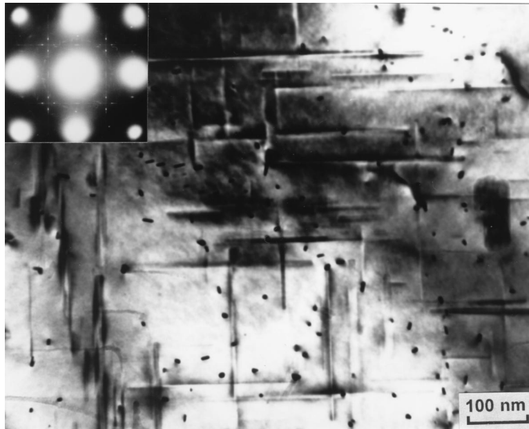
Figure 3. Precipitation morphology ( [001]_{Al} zone axis) of the sample heated to 300^{\circ}\text{C} at 10^{\circ}\text{C}/\text{min} immediately after solutionizing and quenching. At this stage, rod-like and lath-like precipitates predominate.
