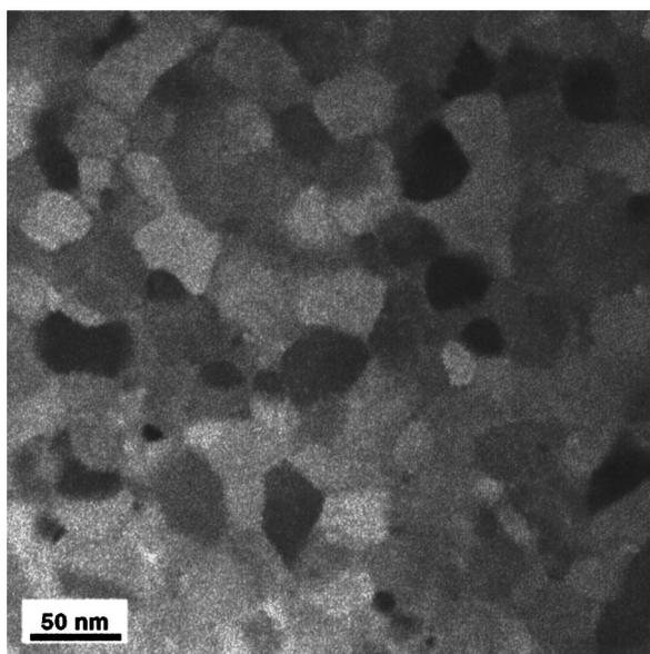
FIG. 1. Bright field image of the NdFeB nanocomposite.
