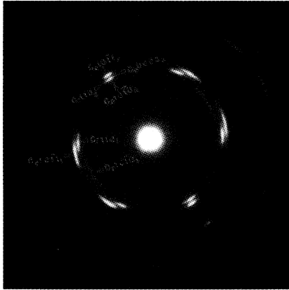
Figure 11. Indexed electron diffraction pattern of (11\bar{2}0)_{\text{CoCrTa}} // (002)_{\text{Cr}} bilayer film at 60^\circ tilt. From (20).
