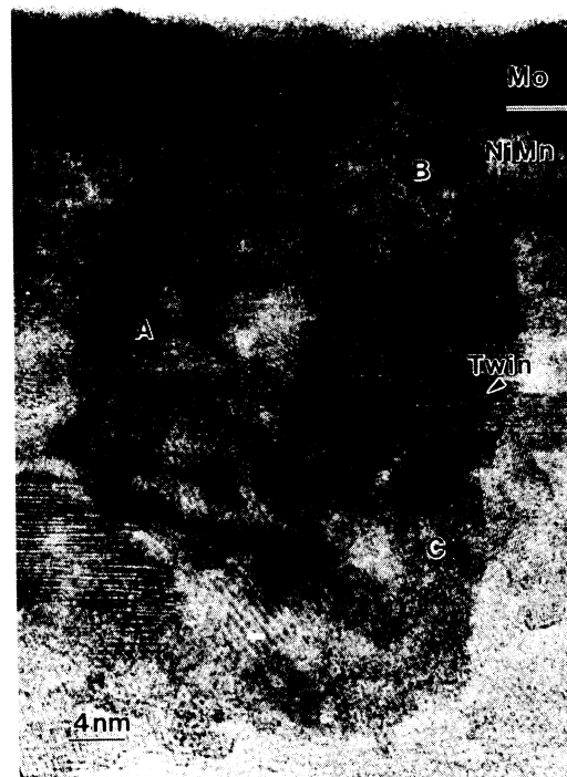
FIG. 18. HRTEM image of a NiMn column in E.
