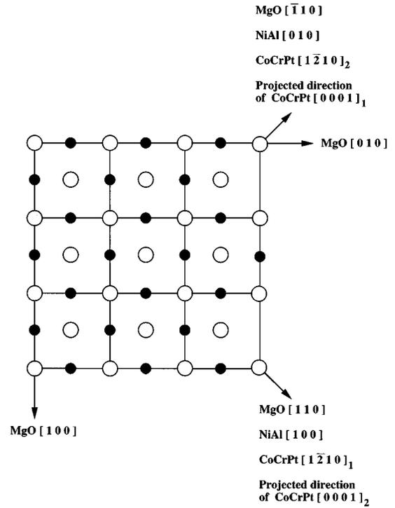
FIG. 4. Directional relationships between those of the CoCrPt/NiAl layers and those of the (001) MgO substrate.
