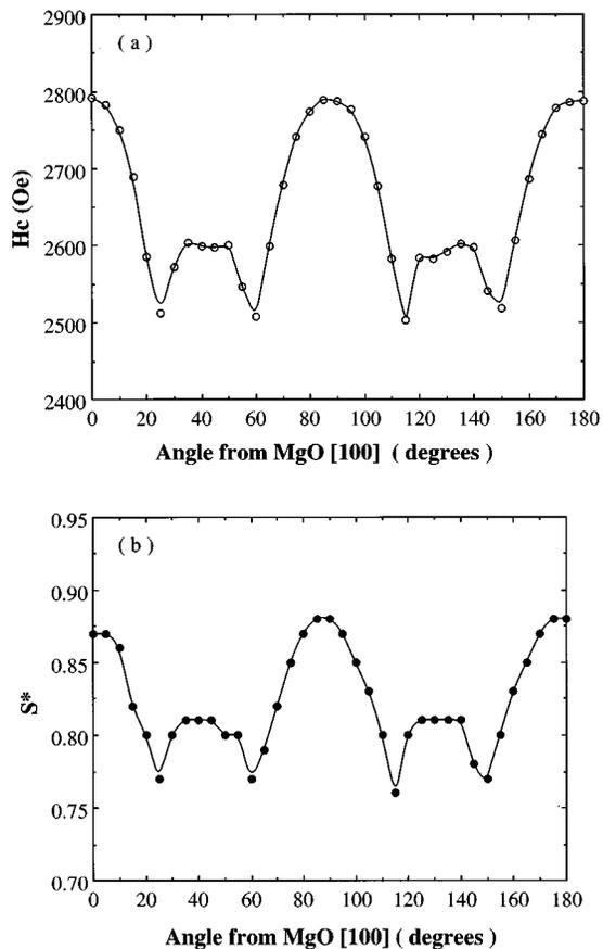
FIG. 5. Variation of (a) coercivity and (b) coercivity squareness of the CoCrPt film with the angle with respect to MgO [100] direction.
