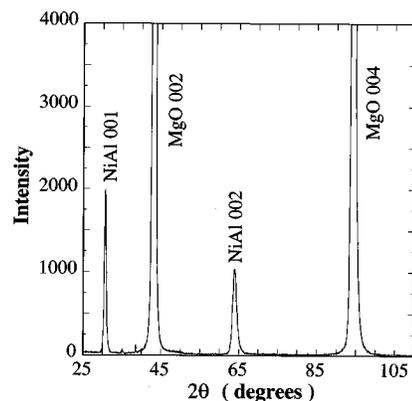
FIG. 1. The x-ray diffraction spectrum of the  $\text{Co}_{72}\text{Cr}_{10}\text{Pt}_{18}/\text{NiAl}/\text{MgO}/(001)\text{MgO}$  film.
