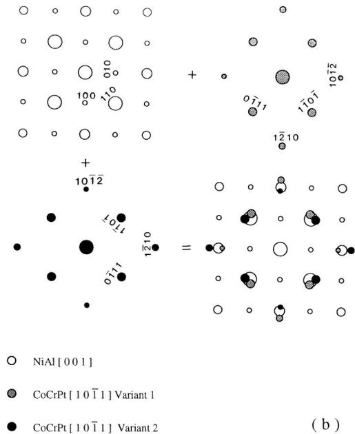
FIG. 3. (a) NiAl[001] zone axis electron diffraction pattern of the CoCrPt/NiAl bilayer, and (b) simulated [1011]CoCrPt/[001]NiAl, and (1210) CoCrPt/(100)NiAl, or (1210)CoCrPt/(010)NiAl, electron diffraction pattern.
