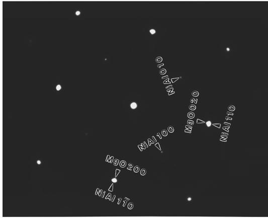
FIG. 2. [001]zone axis electron diffraction pattern of the NiAl/MgO/(001)MgO layers.
