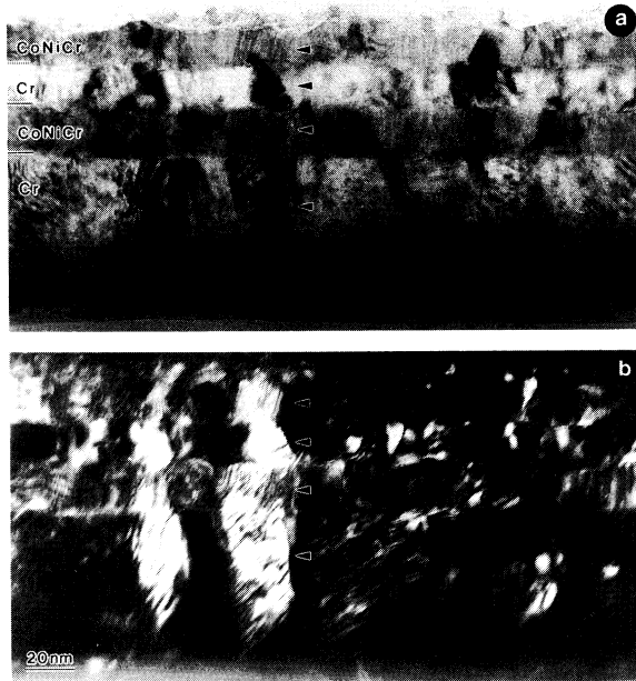
Figure 10. Cross-sectional TEM image of a CoNiCr/Cr multilayer thin film. (a) Bright Field, (b) Dark Field.
