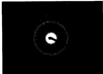
FIG. 4. SAD pattern for sample of unannealed film suggesting an amorphous structure.
