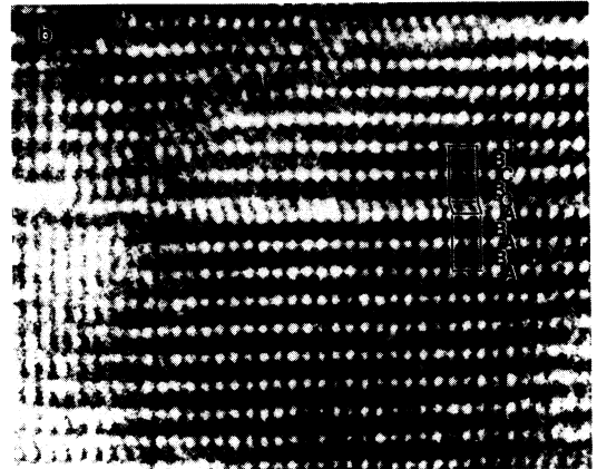
FIG. 4. (a) & (b) HRTEM images of area b and c in Fig. 2. The stacking sequence in both sides of the stacking faults is shown.
