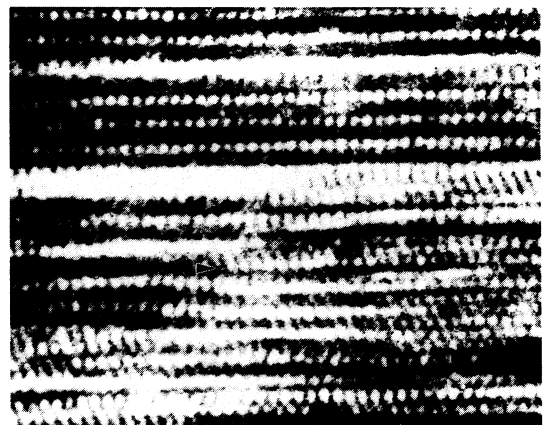
FIG. 5. HRTEM image of area d Fig. 2 showing a SF bounding partial dislocation (arrow).
