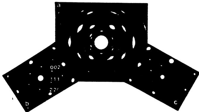
Fig. 3: SAD pattern displays a in-plane crystallographic texture related to the underlying substrate.
