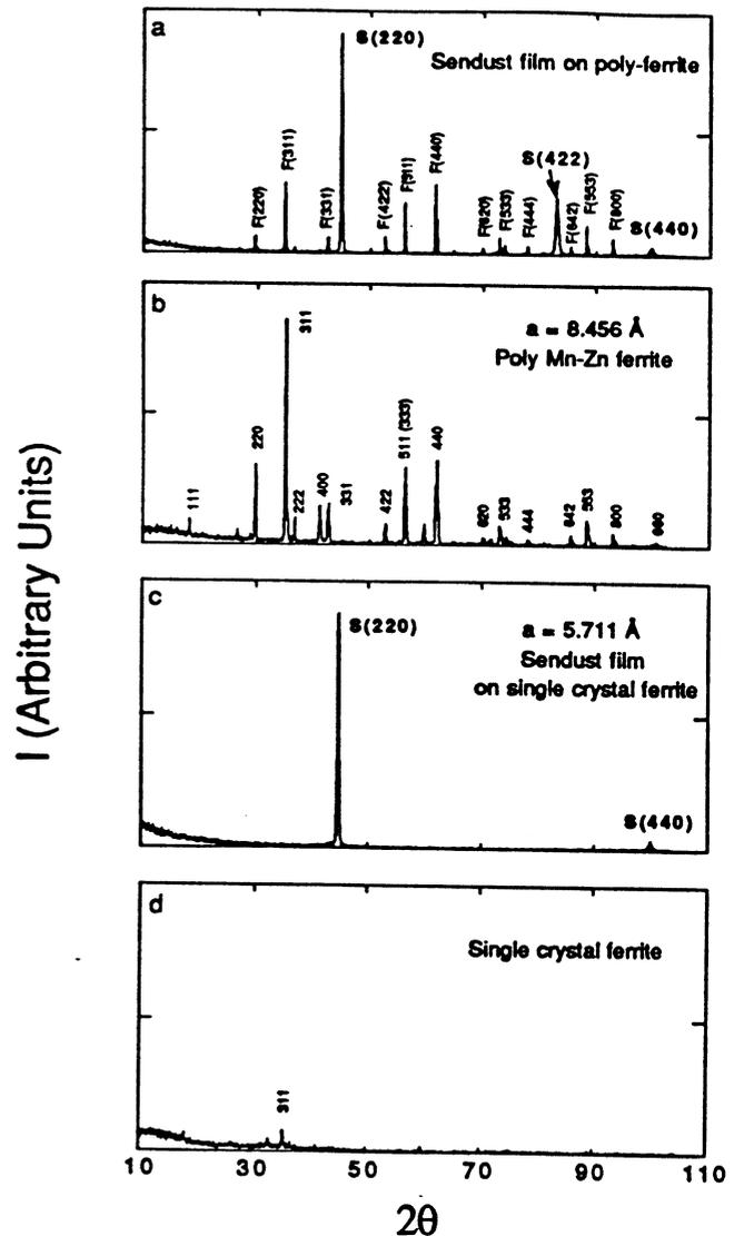
Fig. 2: X-ray spectra showing the out-of-plane {220} texture of the film.
