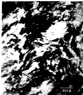
Fig. 4. Heavily twinned PrCo 5 phase.
