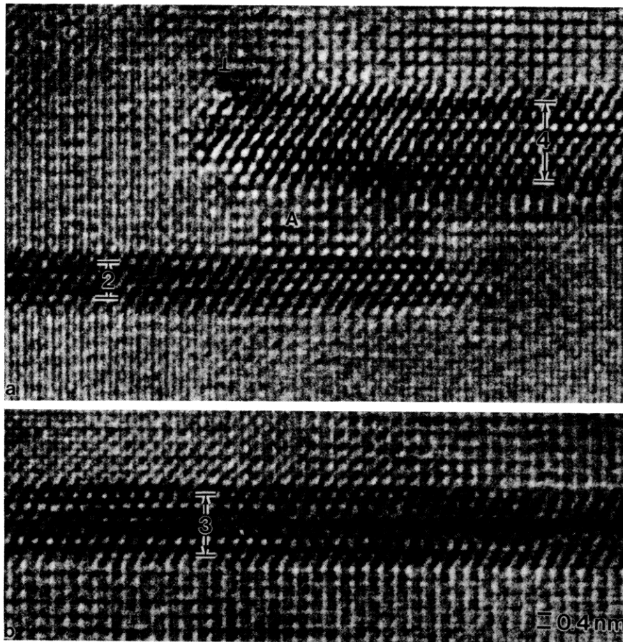
(a) Two and four unit cell \theta' precipitate plates with APBs between \delta' on opposite faces; (b) three unit cell \theta' precipitate with an APB between \delta' on opposite faces.
