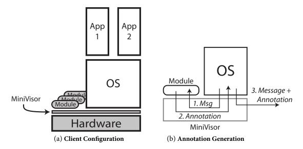
Figure 5.2: **Client Operations. (a)** *The client attests to the presence of a protective layer (MiniVisor) that isolates modules from untrusted code (and vice versa) and from each other. This allows the client to attest to multiple relying parties without a reboot.* **(b)** *Untrusted code submits messages (e.g., email or packets) to the modules to obtain authenticated annotations.*
