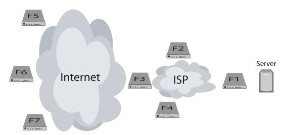
Figure 5.8: Filter Deployment. Initially, a server is likely to deploy a single filter (F1) on its access link. For a fee, an ISP may decide to deploy filters (F2-F4) at its access links. The server may also be able to leverage filters scattered around the Internet (F5-F7) if it has business relations with these entities.
