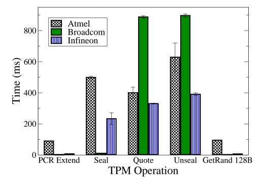
Figure 4.11: **TPM Microbenchmarks.** *TPM benchmarks run against the Atmel v1.2 TPM in a Lenovo T60 laptop, the Broadcom v1.2 TPM in an HP dc5750, the Infineon v1.2 TPM in an AMD machine, and the Atmel v1.2 TPM (note that this is not the same as the Atmel TPM in the Lenovo T60 laptop) in the Intel TEP. Error bars indicate the standard deviation over 20 trials (not all error bars are visible).*
