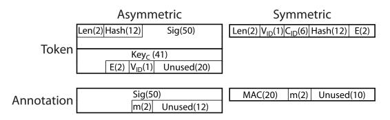
Figure 5.9: Token and Annotation Layout. Byte-level layout for Sender Tokens and traffic annotations. The two are shown separately for clarity, but in practice, would be packed together. E is an expiration date, and m is a randomly-chosen nonce.
