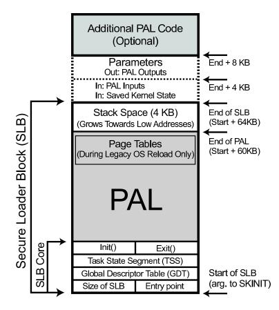
Figure 4.4: **Memory Layout of the SLB.** The shaded region indicates memory containing executable PAL code. The dotted lines indicates memory used to transfer data into and out of the SLB. After the PAL has executed and erased its secrets, memory that previously contained executable code is used for the skeleton page tables needed to reload the OS.
