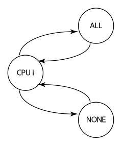
Figure 4.19: **Memory Page States.** State machine for the possible states of a memory page in our proposed memory controller modification. The states correspond to which CPUs can access an individual memory page.
