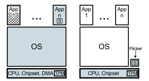
Figure 4.1: **Trusted Computing Base Comparison.** On the left, a traditional computer is shown with an application that executes sensitive code (S). On the right, Flicker protects the execution of the sensitive code. The shaded portions represent components that must be trusted; other applications are included on the left because many applications run with superuser privileges, or with the same user privileges as the application executing sensitive code.
