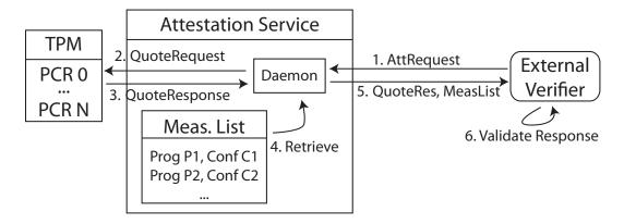
Figure 2.3: Attestation. High-level summary of TPM-based attestation protocol based on signed hash chain measurements [200], e.g., as in IBM's Integrity Measurement Architecture [170]. Some protocol details are elided, e.g., the inclusion of an anti-replay nonce as part of the AttRequest message.
