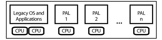
Figure 4.17: Goal of Our Architectural Recommendations. *Physical platform running a legacy OS and applications along with some number of* PALs.
