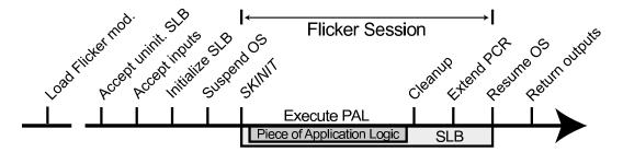
Figure 4.2: PAL **Execution**. *Timeline showing the steps necessary to execute a* PAL. *The SLB includes the* PAL, *as well as the code necessary to initialize and terminate the Flicker session. The gap in the time axis indicates that the flicker-module is only loaded once.*
