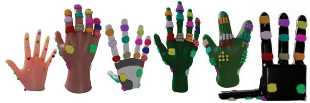
Fig. 5. Single point virtual marker configuration on the source MANO hand and area based corresponding marker sets on all other hands used in our experiments. We use a manifold wrapper of the Allegro Hand for contact processing. Marker points were selected at vertex indices for convenience.
