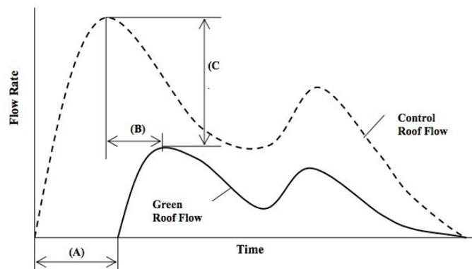
Figure 7: Diagram of Control Roof and Green Roof Runoff Flow-rates [1]
