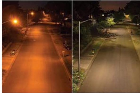
*Figure 15: The image on the left shows a neighborhood street lit with sodium vapor streetlights. On the right is the same street under LED lighting.*
