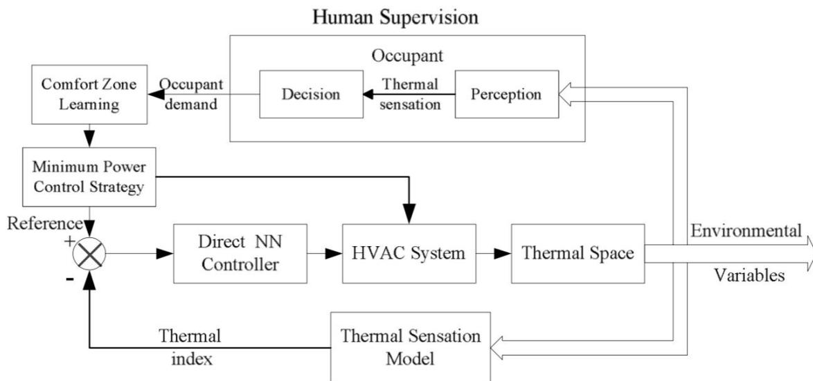
Figure 12: Block diagram of the Thermal Comfort Controller in [43]
